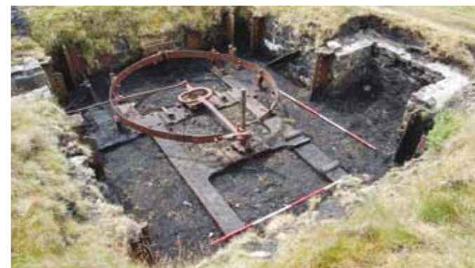
The engine brake wheel – this is an example of a unique mechanism used to slowdown the heavily laden drams on the many tramroad inclines.
